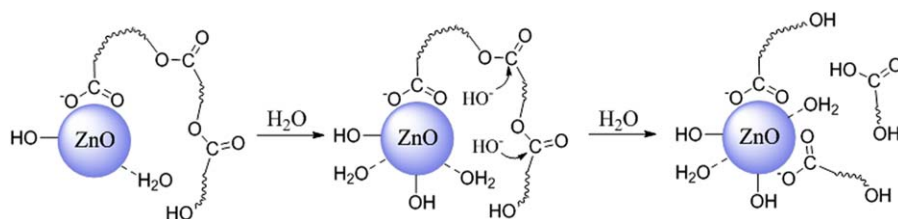
Scheme 1. Hydroxylated ZnO NPs catalyze the rapid hydrolysis of PLA. [Color figure can be viewed in the online issue, which is available at wileyonlinelibrary.com .]
